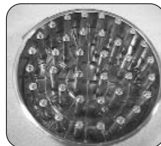
Figure 10: Plugs with Stems are shown when the Divider (fig. 8) is removed. Notice the three different circles of Plugs and the pattern they are in.
