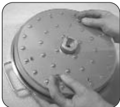
Figure 5: If you wish to disassemble completely, place the Head Assembly into the Pan, loosen both Knurled Knobs and lift off Cover Plate.
