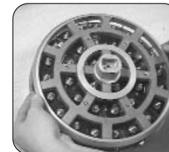
Figure 8: The Divider Assembly may now be removed but need not be disassembled further.
