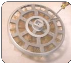
Figure 9: To disassemble the Divider from the Divider Plate, remove the six screws and separate these parts.
