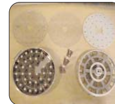
Top L to R: Cover Plate, Locking Plate, Plug Plate Bottom L to R: Pan, Plugs, Divider & Divider Plate
