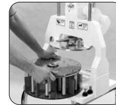
Figure 4: Return the Handle to the upper position and remove Head Assembly for cleaning or interchange with Optional Head Assembly.
