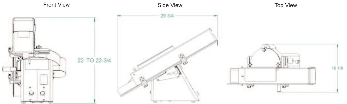
**Capacity: Bun Height: 3" (76mm) Full Cut Width: 4-3/8" (111 mm)**
